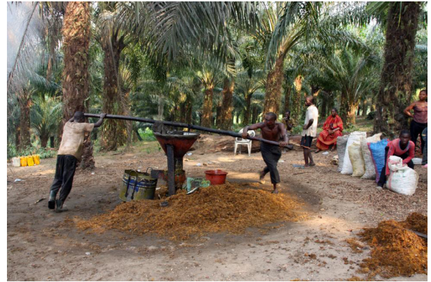
Fig. 5. Palm oil millers in Cameroon use a vertical Caltech expeller in 2013, nearly 30 years after the technology was introduced. Source: Patrice Levang, CIFOR/IRD 2013.
