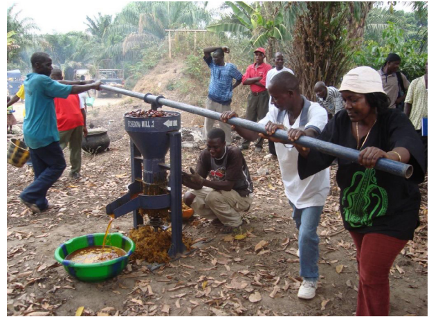
Fig. 1. Promotional demonstration of the vertical Caltech expeller in Liberia; Source: Varney Seasay 2010.
